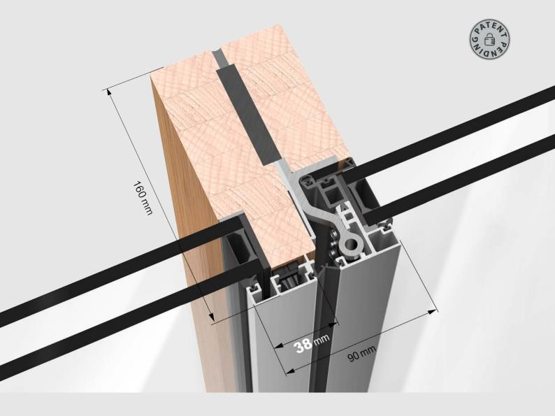
Slim AluClad over wood F38 is a revolution in glazing where minimal timber composite frames can at last achieve a high thermal and acoustic performance.
