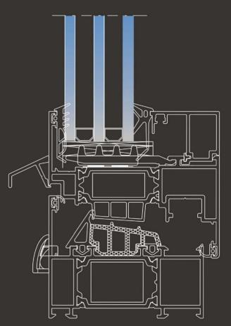
Supreme S77 system is Alumil's latest proposal for advanced insulating hinged systems which meets the high standards of private and public buildings in Western Europe, combining the demanding levels of thermal insulation, water tightness and sound insulation. The system includes a wide range of profiles with modern flat shape, as well as with Alumil's characteristic curved shape.
