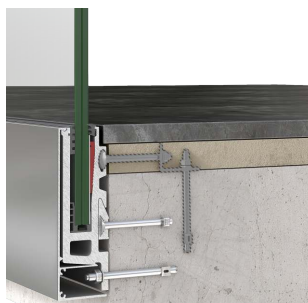
M8202 side-mounted, with 8+8mm and 10+10mm glass
