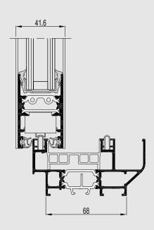
Concept Patio® 68 is a well insulated sliding system that combines elegance with performance and security. This unique sliding system is characterised by its slim profiles, allowing the integration of large windows and doors for maximum views, in combination with burglary resistance class RC2. The integrated innovative technologies guarantee ultimate performances with regard to wind and water tightness and thermal insulation, meeting with the highest standards.
